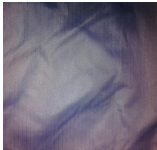
ABOVE YOU SEE A SAMPLE OF OUR FLO-SHIELD ESD BARRIER FABRIC WITH CARBON FIBERS TO PREVENT STATIC BUILDUP.
